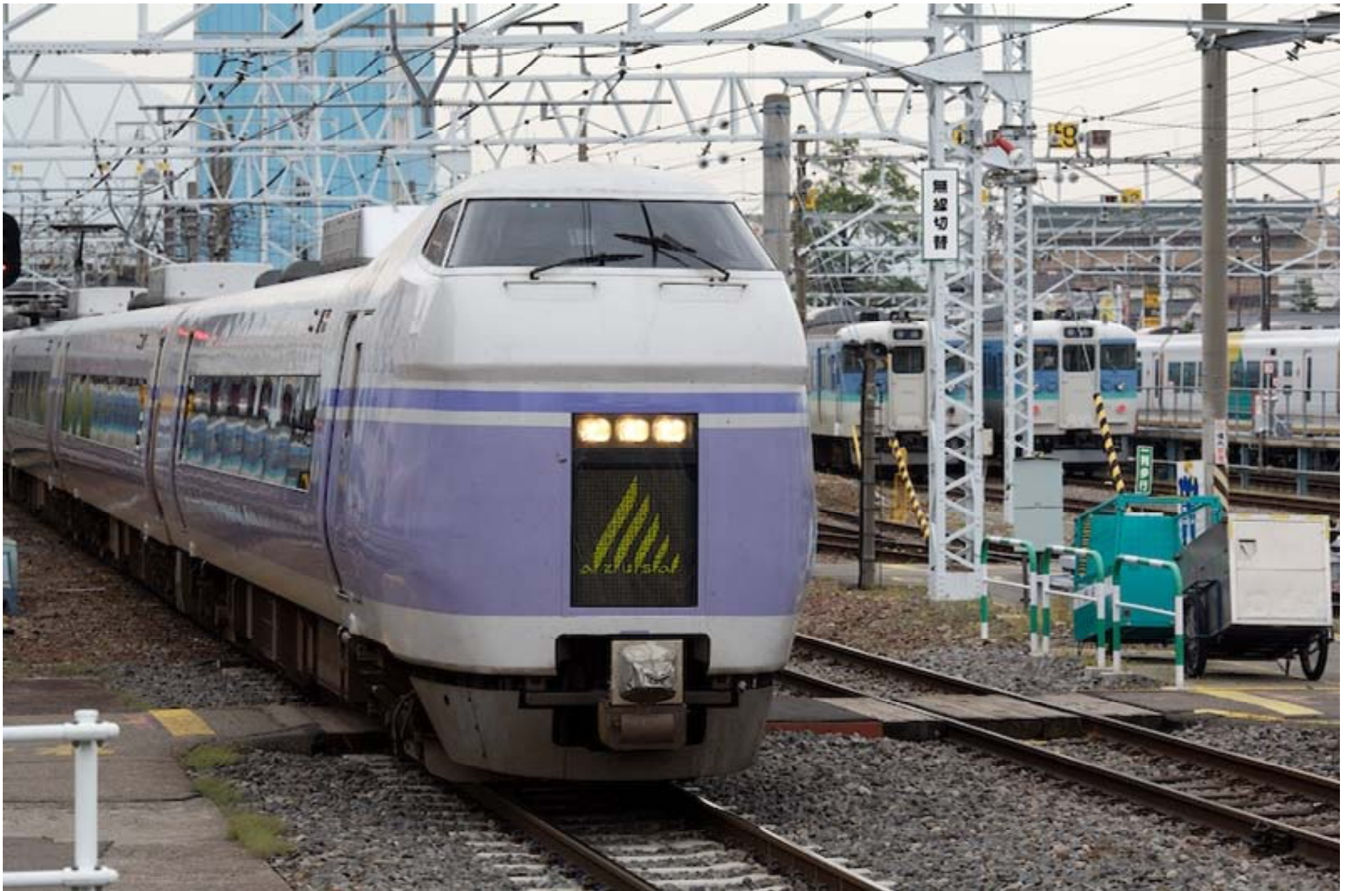
JR East narrow gauge Super Azusa Limited Express tilting EMU train at Matsumoto on the Chuo line to Tokyo.
